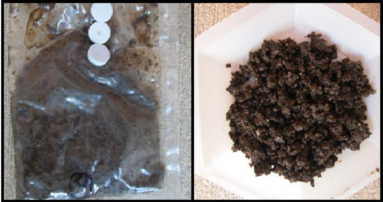
Figure 4-9. Picture of compost plus PLA after 40 days, in and out of the bag
