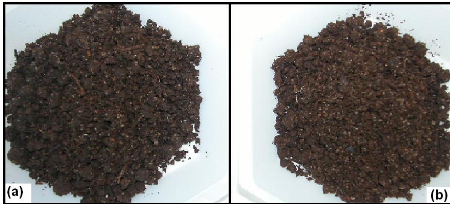
Figure 6-5. Biodegraded PLA in compost: (a) compost by itself, (b) compost + PLA (not seen any more)
