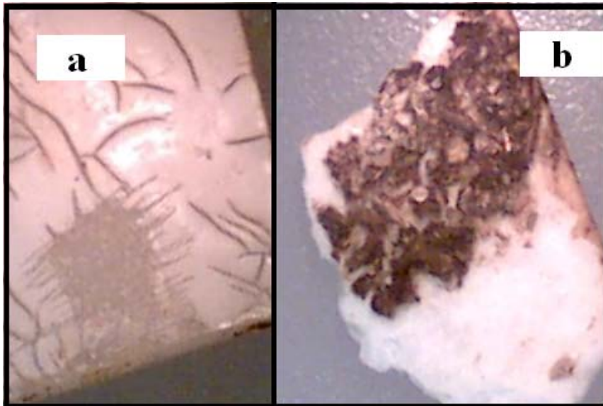
Figure 2-12. Structural integrity of e-beam irradiated/composted PLA: (a) early cracks affecting surface, (b) layer formation and overall structure affected
