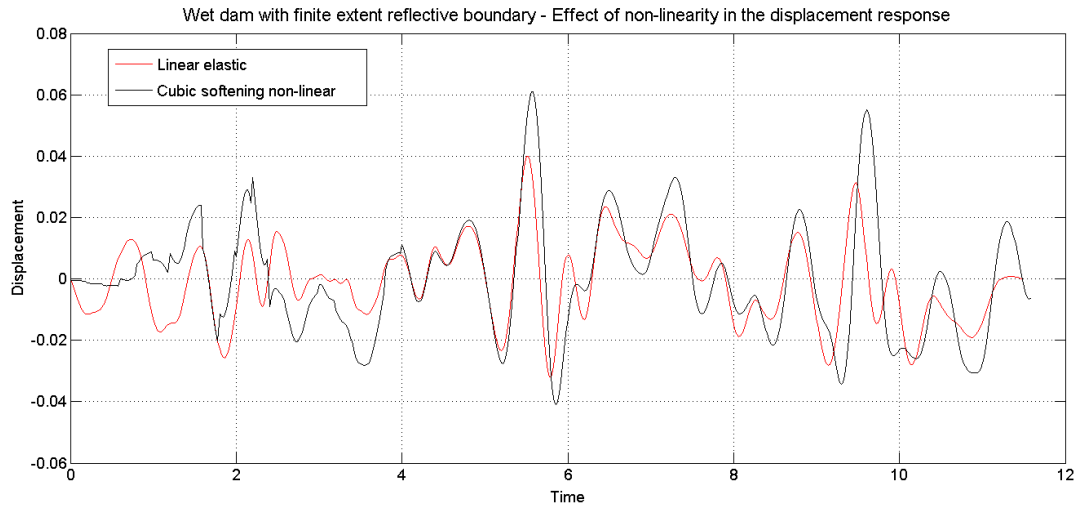
Figure 6.16: Dam-reservoir interaction with finite extent reflective boundary (Case II). Effect of non-linearity in the displacement response.
