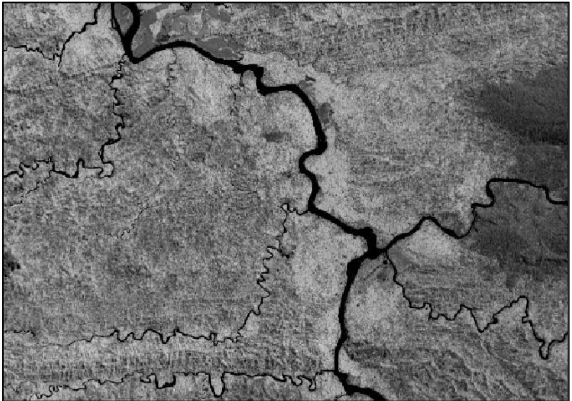
Figure 18: NDVI of the SPOT image, for comparison with classified image. Lighter areas depict more vigorous vegetation.
