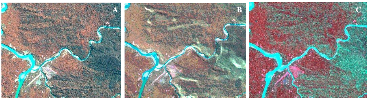
Appendix 3, figure 3: Image normalization for relief shade. Picture A: original SPOT image (B2,B3,B4). Picture B: Topographic normalized image (using DEM created from contour lines). Picture C: Equal area normalized image.
