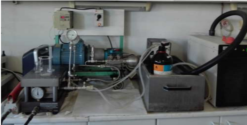
Figure 3.2 Photograph of the nanofiltration system with membrane MPF 36
