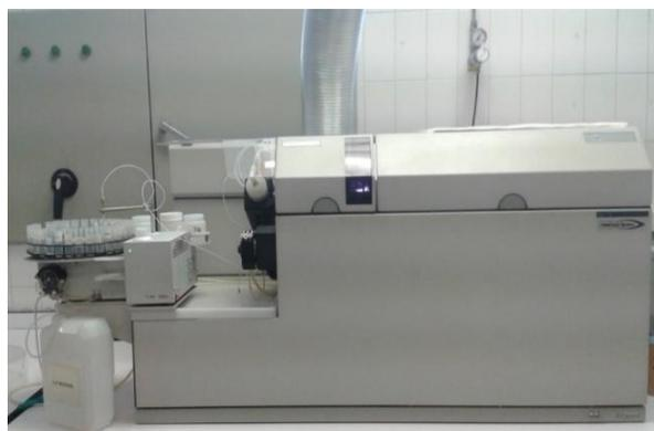
Figura 3. ICP-MS - Agilent 7500a
