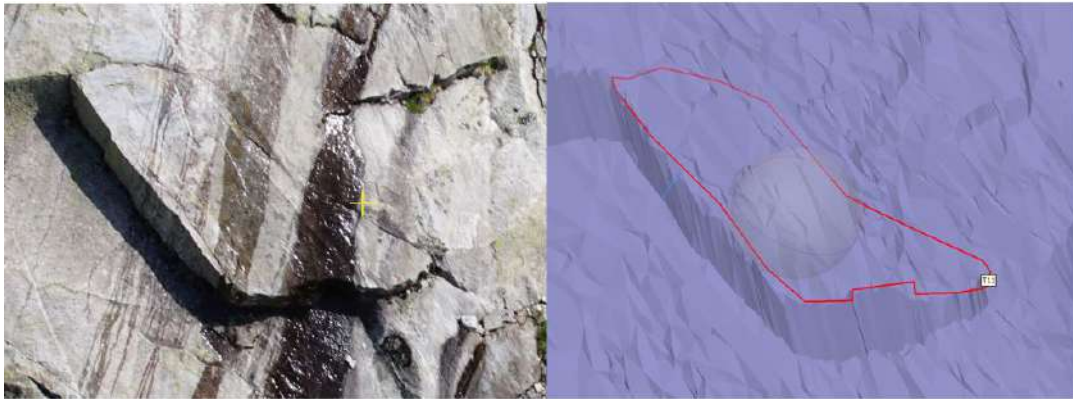
FIGURE 4.12: On the left, you can observe the single block with the presence of a fracture at the top. On the right side the DEM of the proposed block in red.
