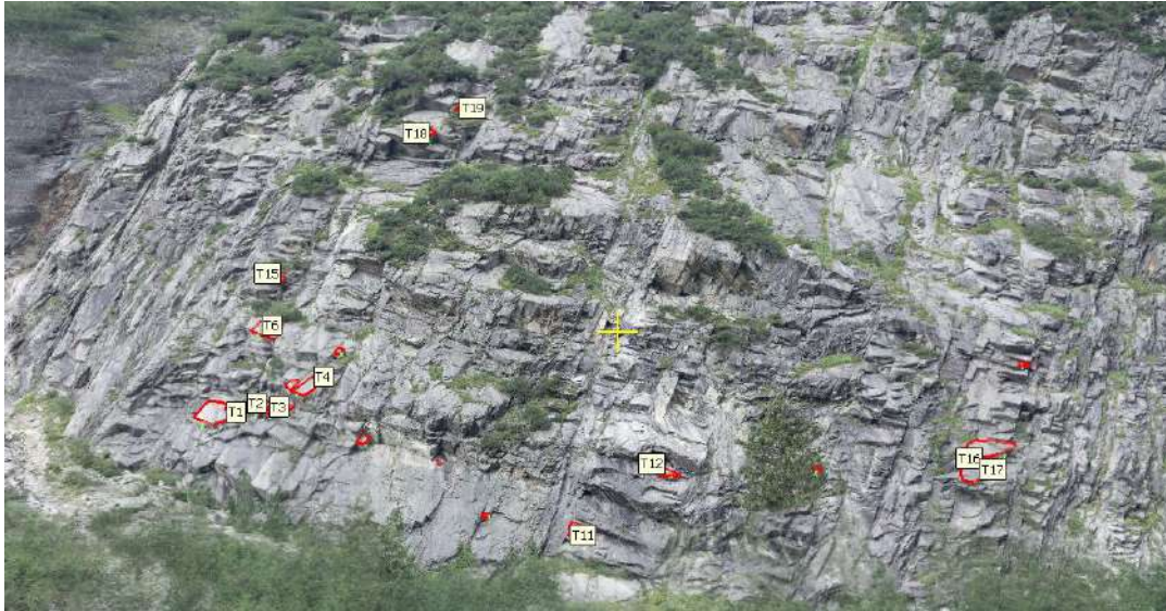
FIGURE 5.10: Tschingelmad, the red polygons are the existing blocks. In the area failed blocks were not mapped due to non-recognizable characteristics.
