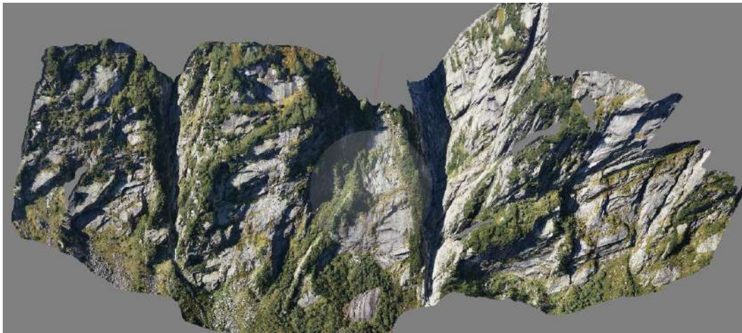
FIGURE 5.8: Photogrammetry of the area denominated Handegg, was performed with a UAV.
