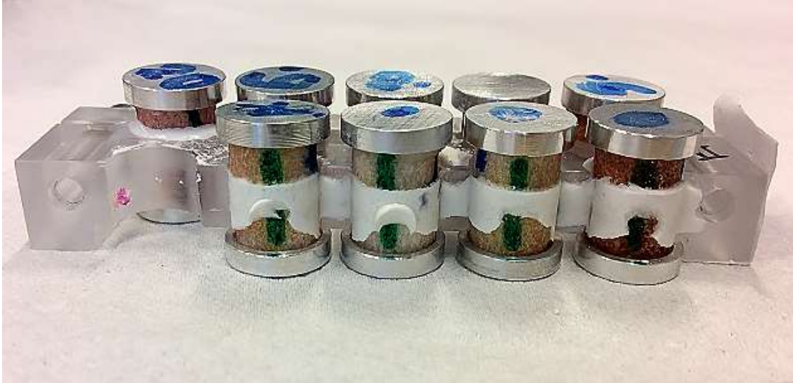
Figure 3. Cemented samples after removal from the customized cement application holder.
