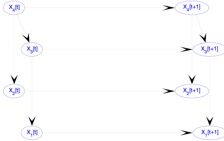
Figure 5–10: Dynamic structure learned of the DBN_{SWaT} model in timestamps t and t + 1 .
