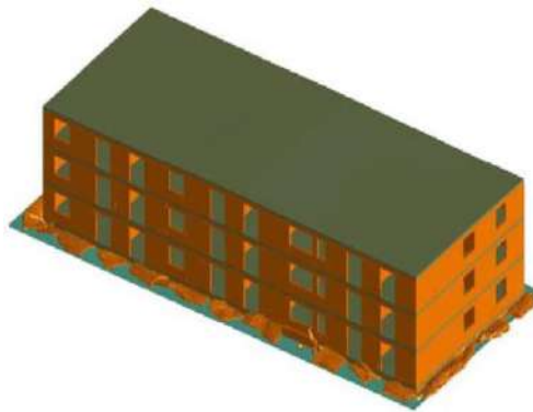
Figure 2.18 Masonry building exhibiting soft storey collapse mechanism, modelled in Extreme Loading for Structures [102] software
