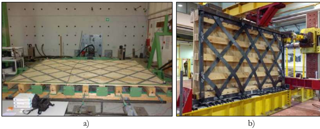
Figure 2.37 Seismic retrofitting of timber slab a) steel strips at top, b) steel strips at bottom [124]
