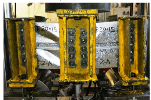
c) Shear failure mode of a purlin with longitudinal web stiffener and aspect ratio of 1.0, SWC-R20 × 15.
