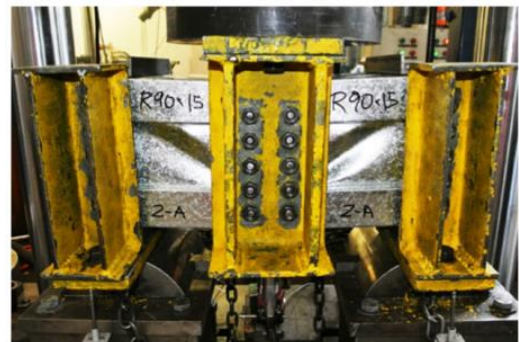
b) Shear failure mode of a purlin with longitudinal web stiffener and aspect ratio of 1.0, SWC-R90 × 15.
