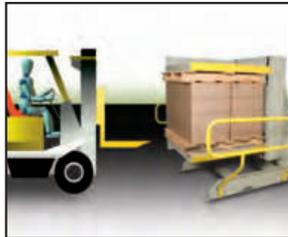
2. Place loaded pallet into rotator/inverter.
