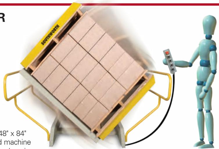
With the ability to handle pallet loads measuring up to 48" x 48" x 84" high, the PalletPal® Pallet Rotator/Inverter is a simple, rugged machine designed to invert entire pallet loads. The pressure adjustable clamping mechanism easily secures loads up to 4,400 pounds and rotates them 180 degrees on a massive anti-friction turret bearing.
