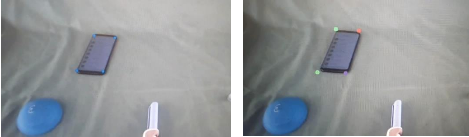
Figure 8: (left) Initial guess of device coordinates (right) Approximation of coordinates in the next frame using the Lucas-Kanade Algorithm.
