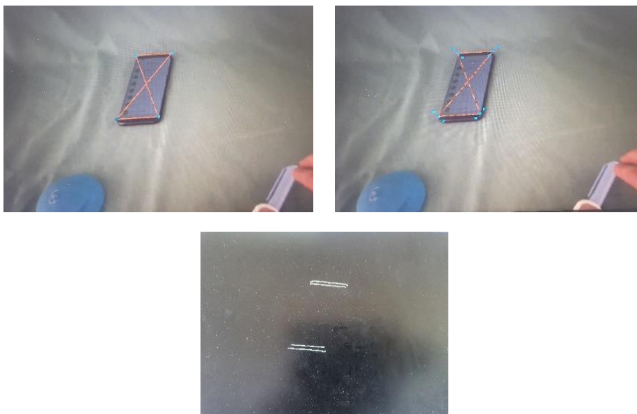
Figure 26: (Upper row) Search area identification after ignoring the is_ok_location checkpoint. (Lower row) Line detection with Canny filter with the respective search area.
