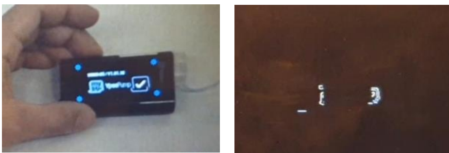
Figure 19: (left) screen coordinates for Ypsopump evaluation and (right) detected lines after the Canny Filter was used
