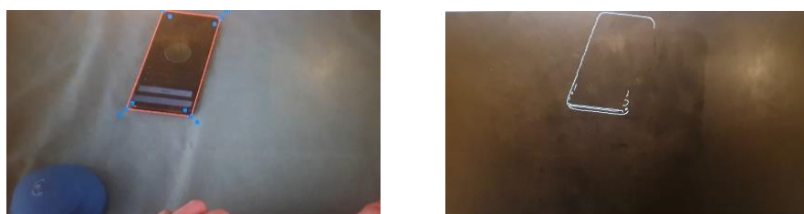
Figure 22: (left) evaluation of Smartpilot app and (right) detected lines with Canny Detector filter
