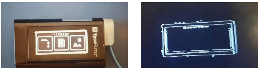
Figure 20: (left) evaluation of Ypsopump with tape and (right) detected lines with Canny Detector Filter
