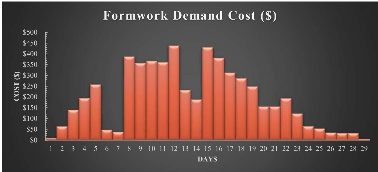
Figure 4.22. Formwork demand profile
