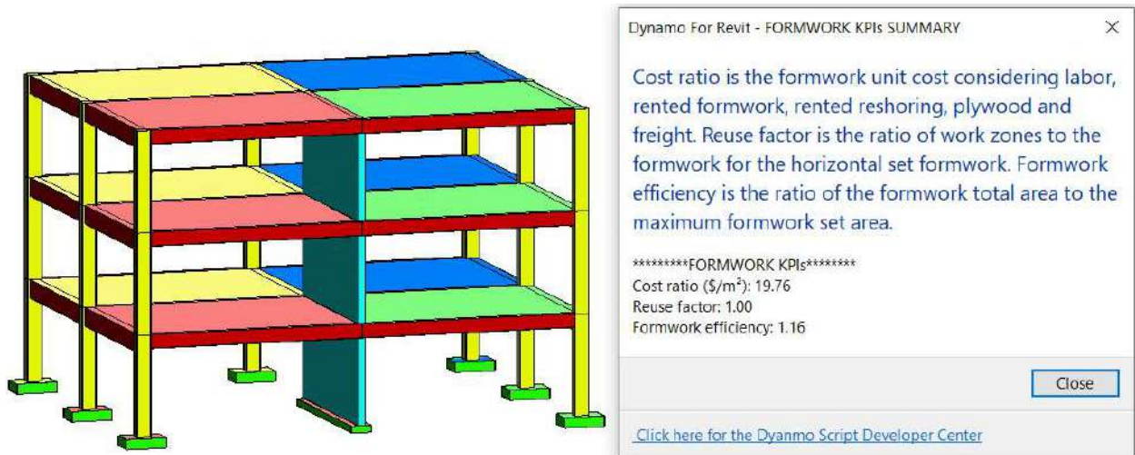
Figure 4.15. Results of running Dynamo script for computing KPIS.
