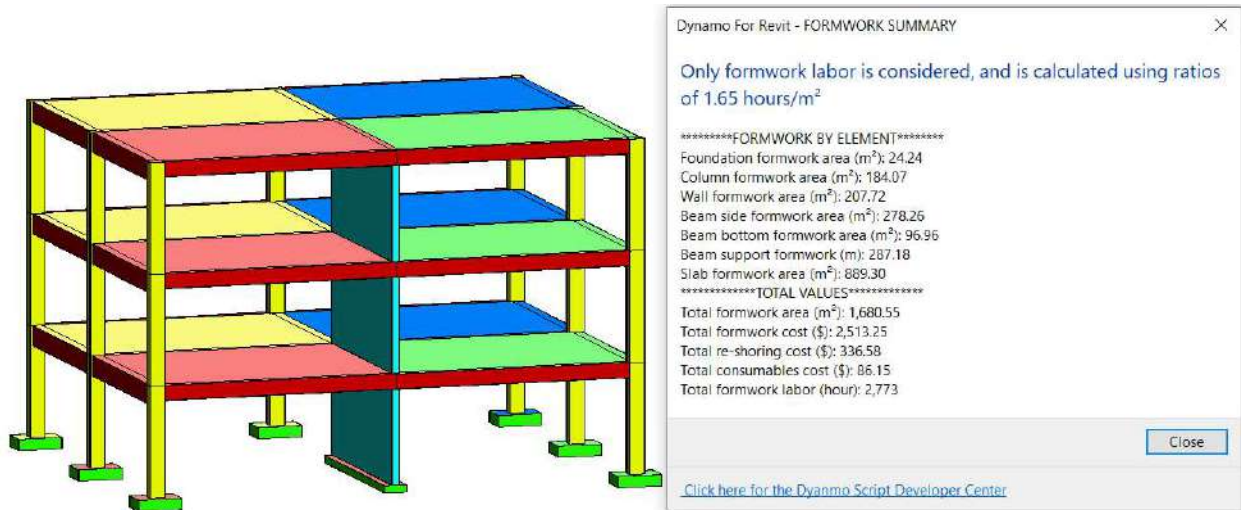
Figure 4.8. Dynamo script for generating formwork summary.
