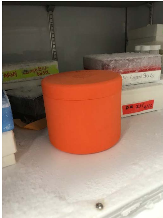
Figure 5. Mr. Frosty device used in the standard freeze procedure. Cryovials are inserted into the styrofoam container that then insulates it from the freezer. This regulates the sample to not experience shock from freezing too quickly, as it decrease by approximately -1^{\circ}\text{C}/\text{min} .
