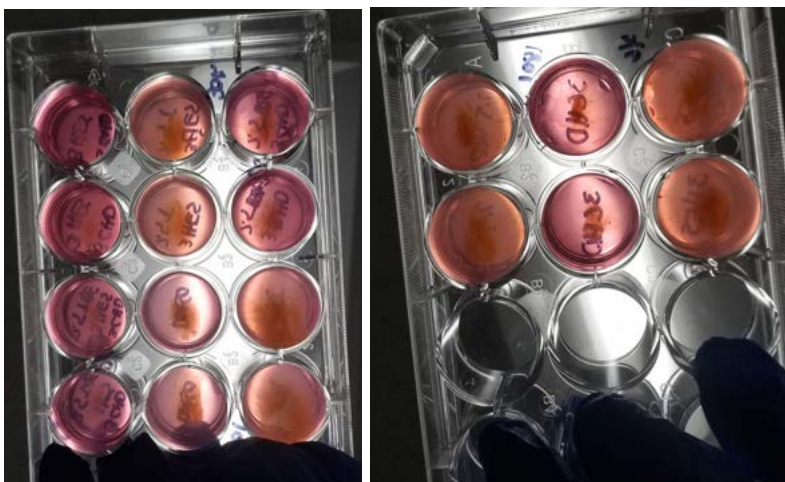
Figure 20. Contaminated wells for the cytotoxicity test. The color difference between the wells shows the contamination present in Trial 2 of the cytotoxicity tests. The oranger wells are the ones that contaminated media was used in and the pinker wells are the ones that contain CHD and did not get contaminated.
