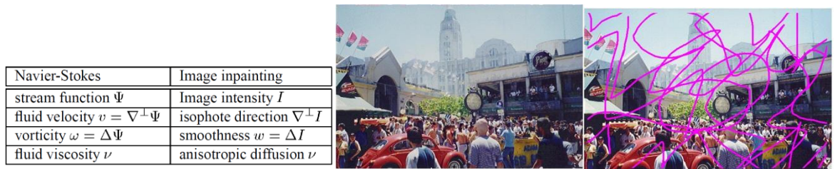
Figure 4-10. (a) Comparative table on the implemented ideas [12] (b) Result of the algorithm [12]
