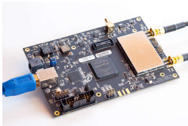
Figure 3.1 Nuand bladeRF transceiver board used in the transmitter.[www02]
