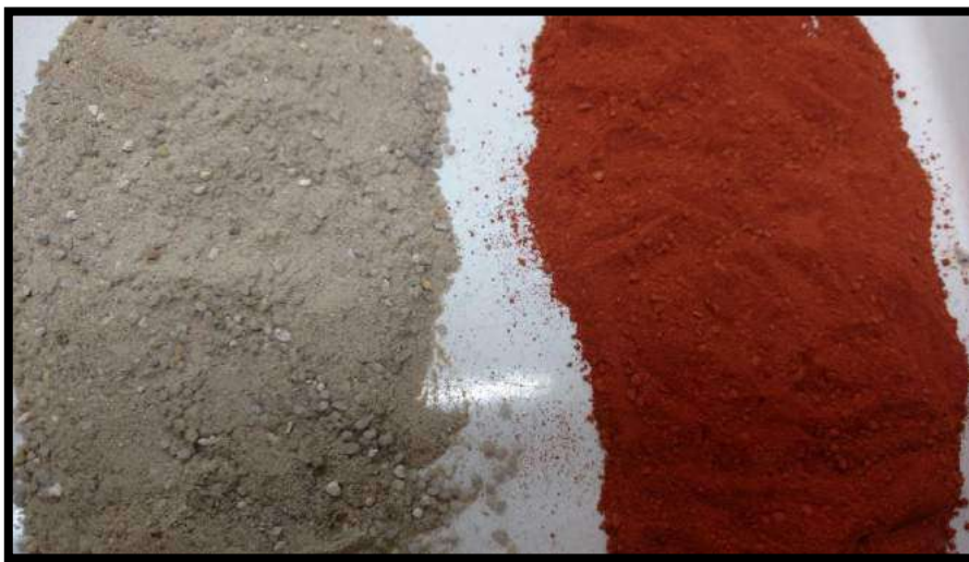
Figure 3.24 Silica Sand Mixture and Adjusted Bauxite
