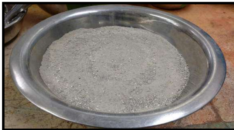
Figure 3.15 Mixture of Silica Sands resembling adjusted Bauxite gradation
