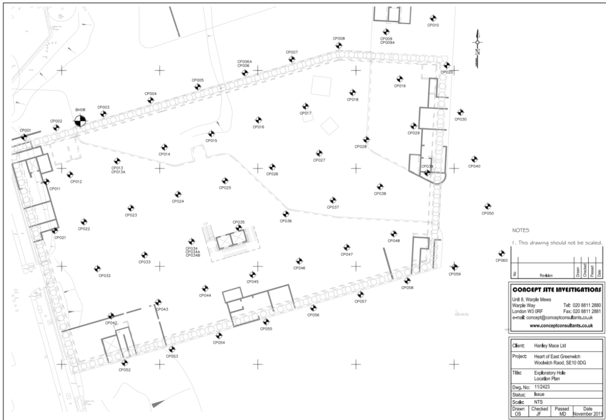
Figure 2.8: Plan view of CPT and Piezocone tests at the Heart of East Greenwich (Savvidou, 2012)
