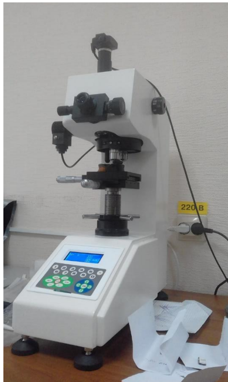
Figure 2-9: the "DM2A" brand Vickers hardness tester.
