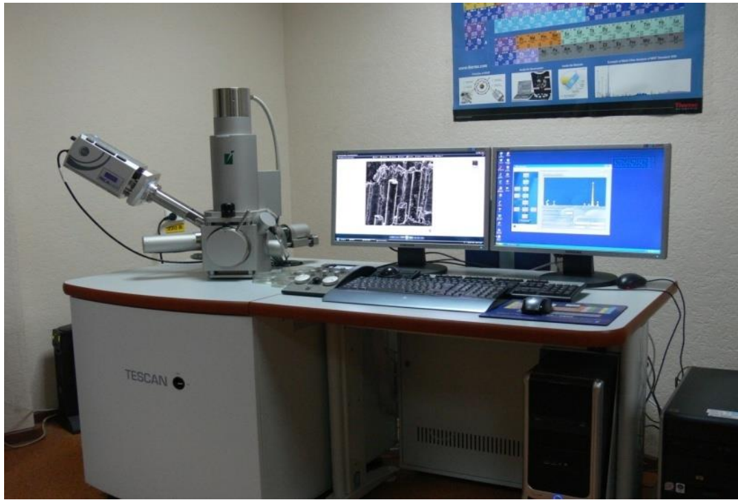
Figure 2.7 - TESCAN Vega SB electron microscope with X-ray microanalyzer INCA
